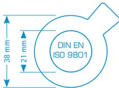
All OCULUS trial frames are suitable for trial lenses conforming to DIN EN ISO 9801 with a rim diameter of 38 mm, e.g. an OCULUS "tl" trial lens
